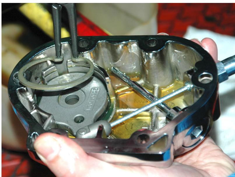
... remove the retaining clip carefully.
